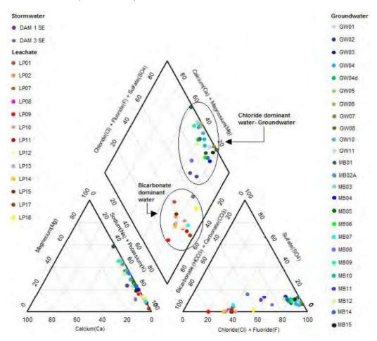
Figure 7-3: Piper Plot - Leachate, Stormwater and Groundwater. April-May 2014 (AECOM, 2016)
