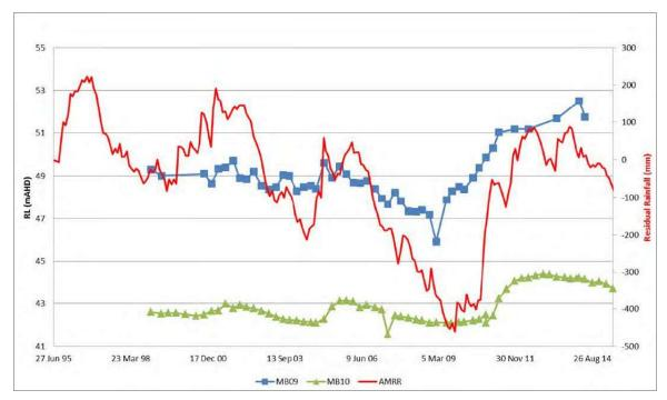
Figure 7-1: Groundwater Elevations in Lower NVA (AECOM, 2016)
