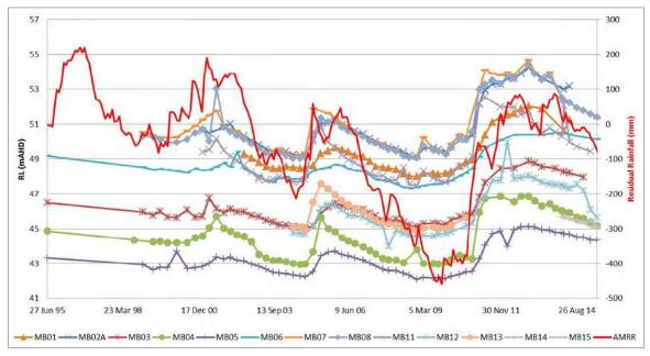
Figure 7-2: Groundwater Elevations in Upper NVA (AECOM, 2016)
